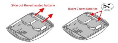
ATTENTION: Use only CR2032 type batteries, different type batteries can seriously damage the sensor. Discard used batteries properly in special dedicated containers.
