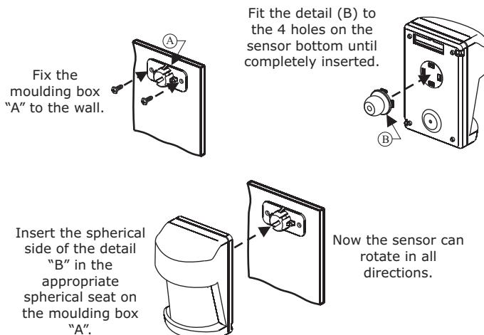
Adjust the sensor taking into consideration the area to be protected and make some functioning test.
