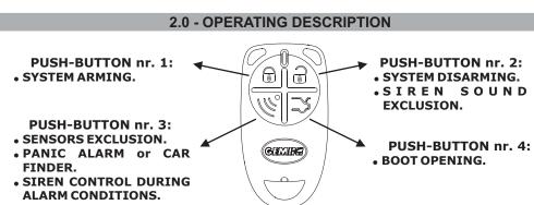
When batteries are almost uncharged, the LED will flash at every pressing of the radio control push button.
